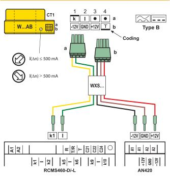
The connections k and l at the residual current monitor must not be interchanged.
